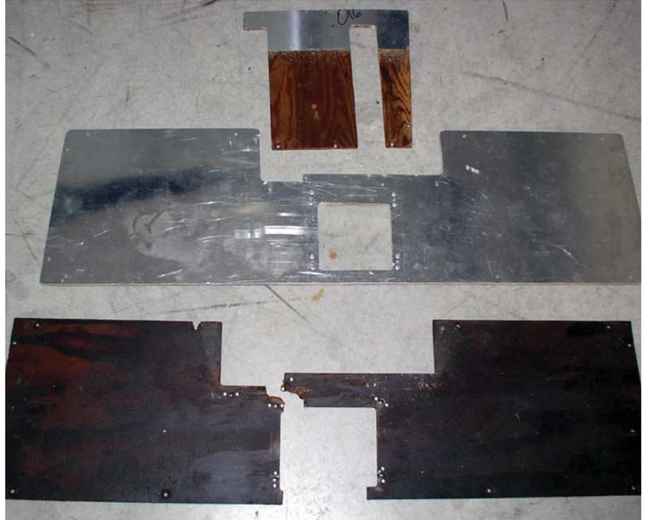
Damaged and flammable, oil-soaked floorboards (at bottom) and new composite floorboards (at top).
