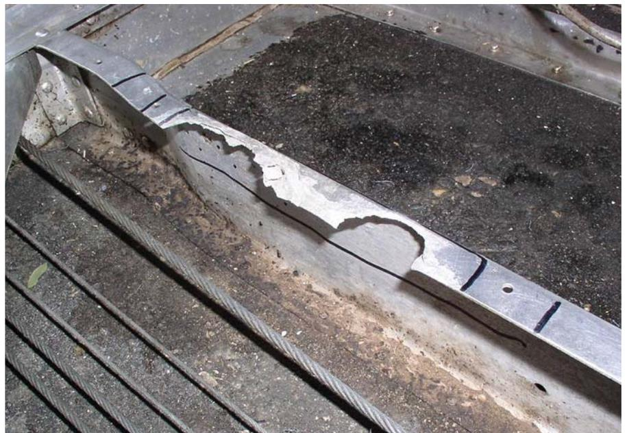
Corroded floor structure and dirty belly.
