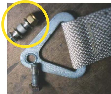
Improper seat belt attachment hardware—correct aircraft structural hardware and spacer shown in upper left circle .
