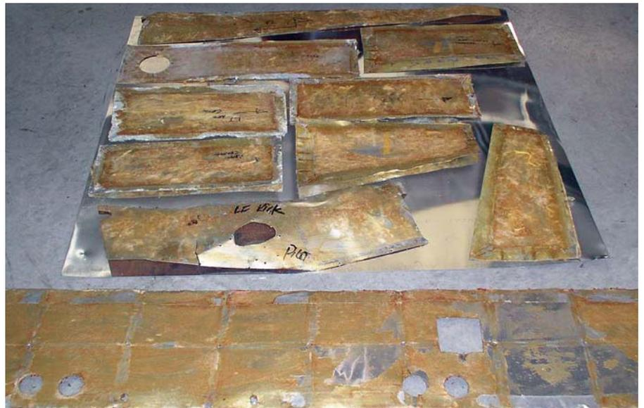
Damaged side panel backing panels.
