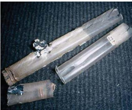
Deteriorated and poorly repaired fresh air ducts.
