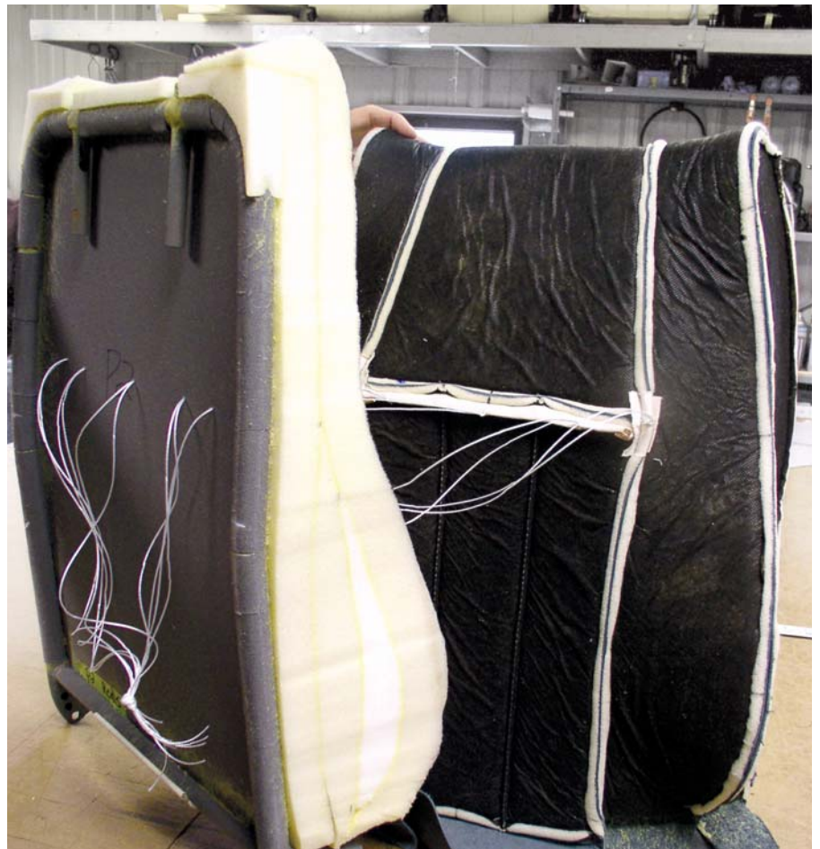
With rigging loosely in place, the seat cover is now ready to turn right side out and pull over the foamed frame.
