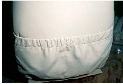
Improperly secured map case, pulling at the sides of the seat.
