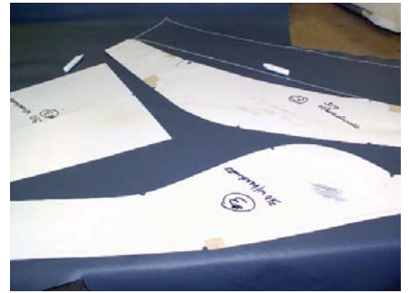
Laying out the patterns on the finish material before cutting.
