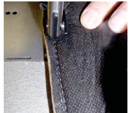
Vertical side section of the seat being sewn on using a cording foot. Note the double stitching.
