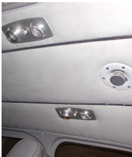
Rail-mounted three-piece headliner with overhead lights and air vents in a B35.
