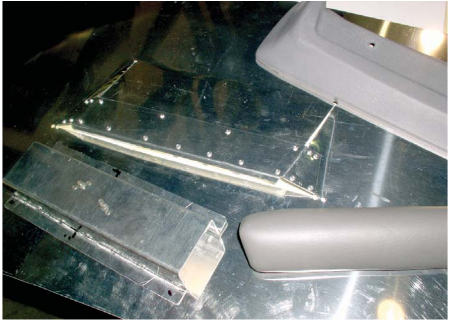
Structural bracket and recession in the side panel to accommodate the new molded armrest.
