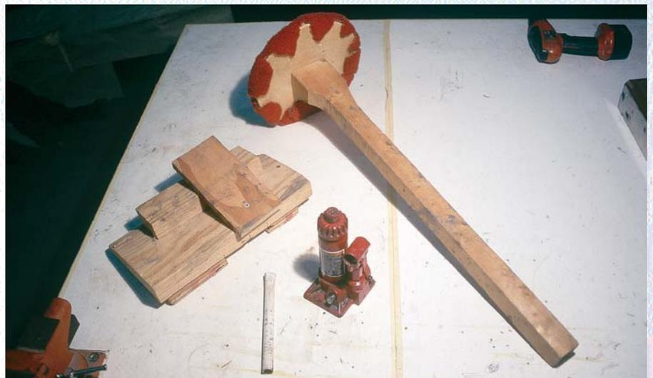
Homemade rail and wood base used with the small bottle jack to lift/push the new windshield into place.
