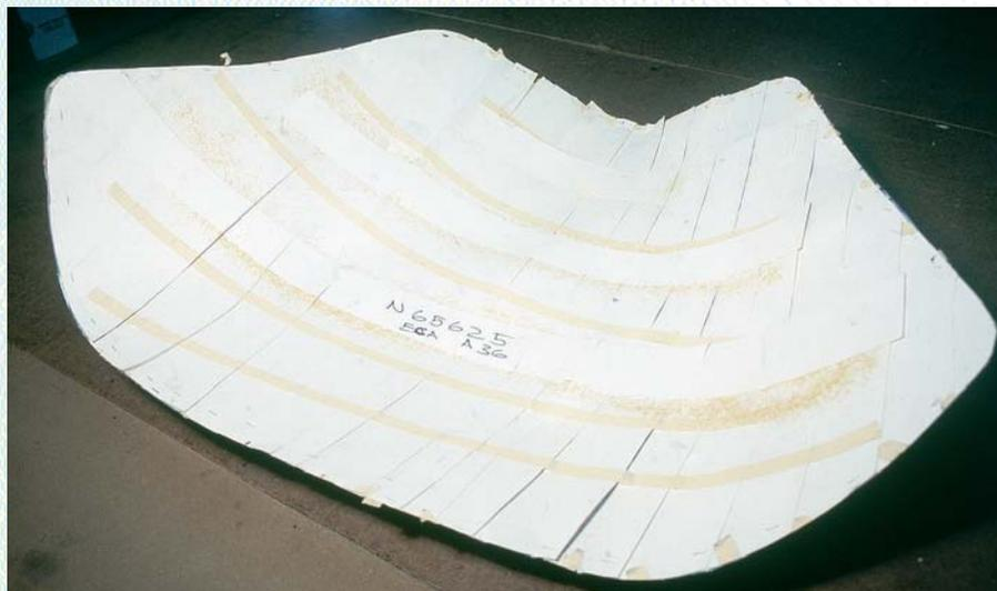
Compound-shaped pattern of original windshield, made from strips of pattern paper.
