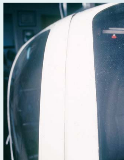
Misaligned cabin doors caused by improperly trimmed windshield being forced into its structural frame.
