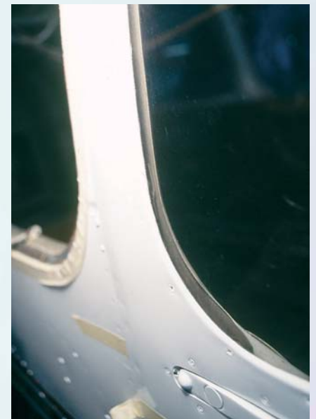
Frameless window installed without the outer trim strip, exposing the backside of the inner window frames and related hardware—very ugly!
