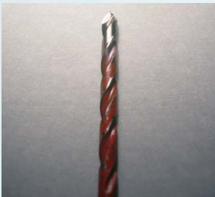
Special tip of Plexiglas drill bit.
