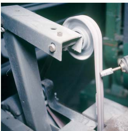
Using a belt sander to round off the cutting flutes of a rotary file.
