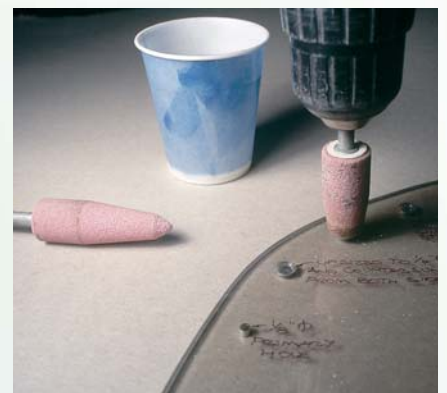
Finishing stones in use to polish the countersunk holes.
