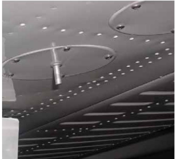
OAT probe mounted in an inspection panel just outboard of the left landing gear on a V35B, shaded from sun and away from any heat source.
