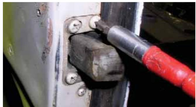
Adjusting the aft door latch bolt mechanism.
