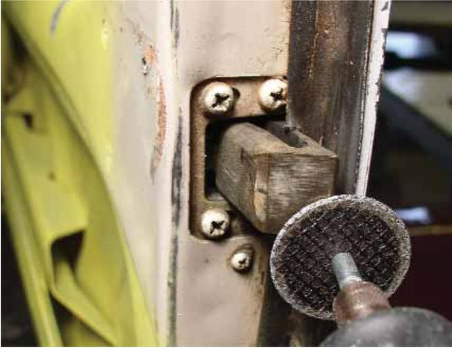
Dressing the aft edge of the door latch bolt.
