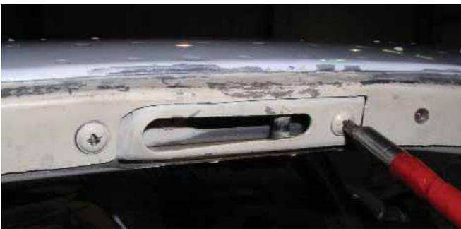
Adjusting the upper door latch receiver.
