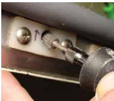
Using a router bit and a moto tool to taper the latch pin receiver.
