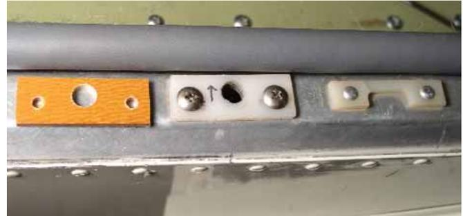
New stronger phenolic latch pin receiver plate on left.
