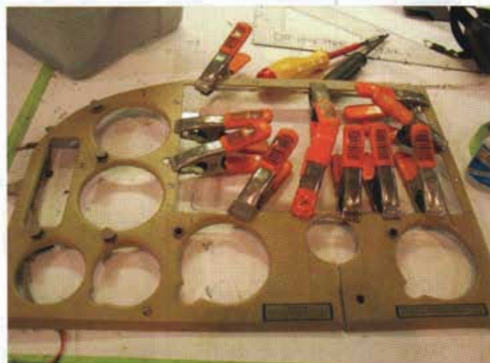
1/4" acrylic doubler being bonded to the original plastic overlay.
