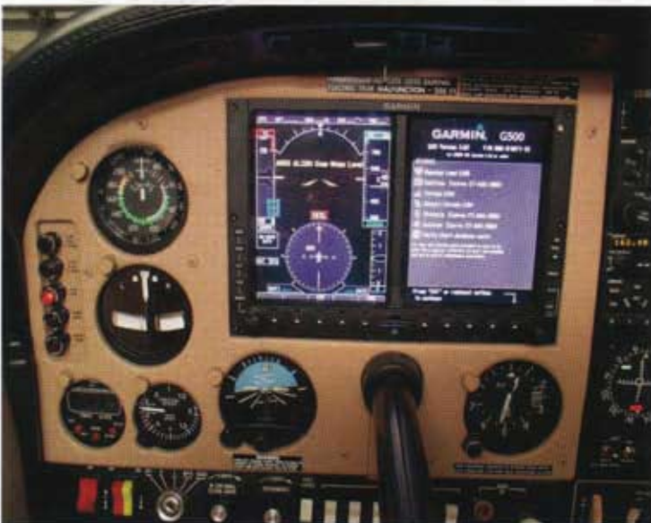
Close-up of the renovated panel with the Garmin 500 installed.
