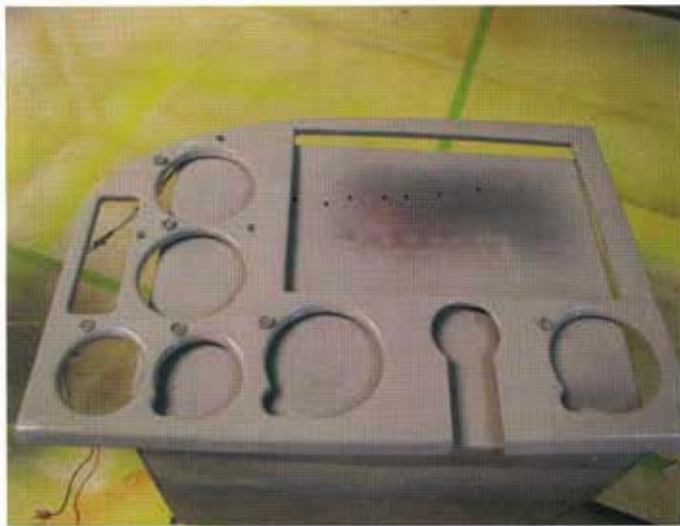
The panel overlay is sanded, filled, primed and ready for paint.
