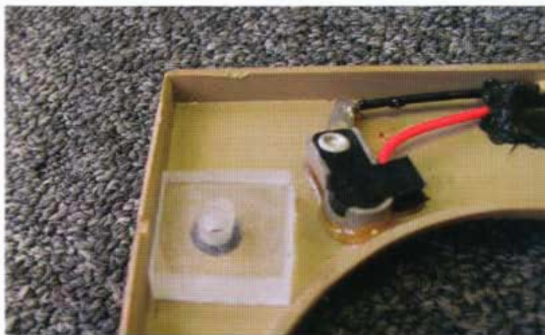
1/4" acrylic mounting screw doubler bonded to the back side of the panel overlay.
