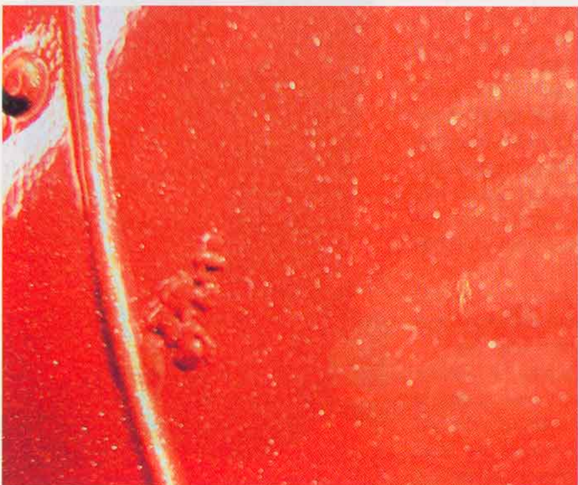
Figure 3—Early stage of filiform corrosion. Notice irregular swelling caused by corrosion trapped under the paint.
