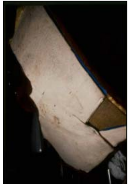
Even the backsides of the forward upholstery panels have damping materials bonded to them.
