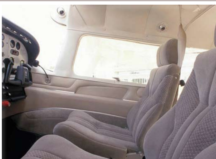
Aluminum rail-mounted continuous armrest with separate pan-type recessions at each seat.
