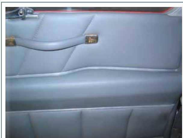
Continuous armrest mounted with contoured aluminum rails that create a phantom recession.
