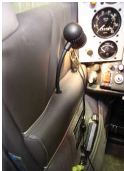
Reading light and mic & phone jacks are nicely installed in a continuous aluminum-mounted armrest.
