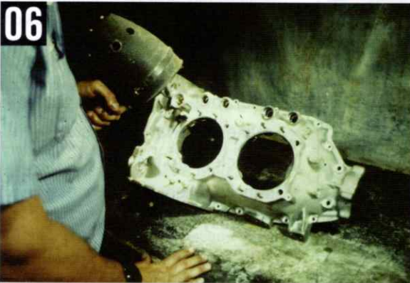
Using a black light to check for cracks in the crankcase.
