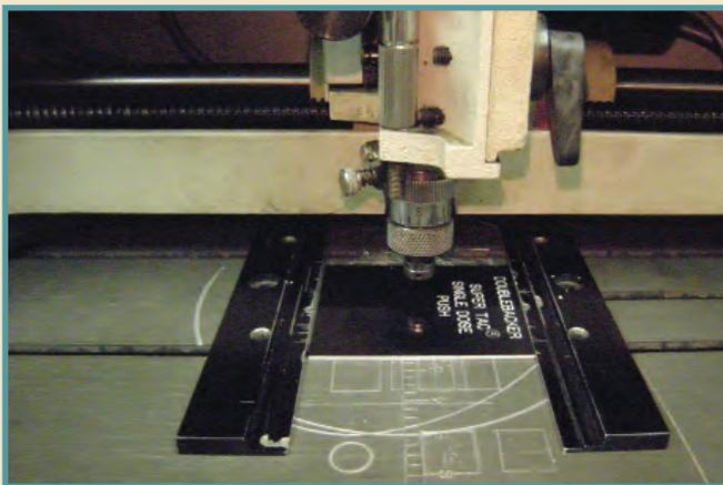
A computer-controlled cutting router.
