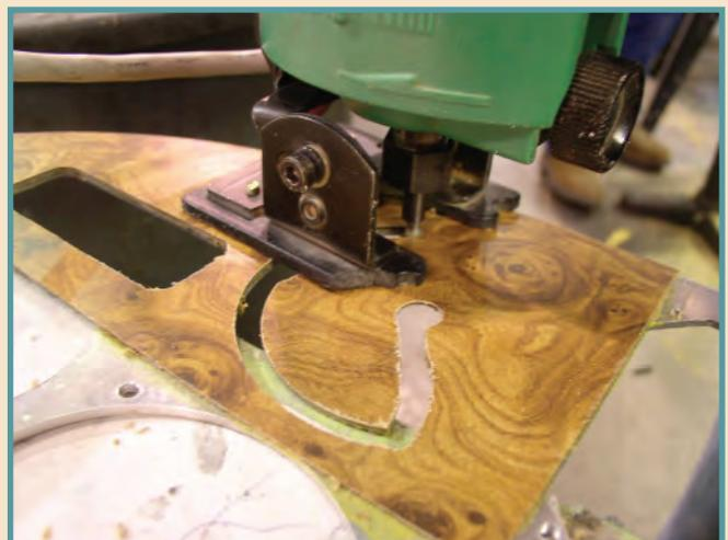
Routing instrument holes in a laminate-covered .090" panel.
