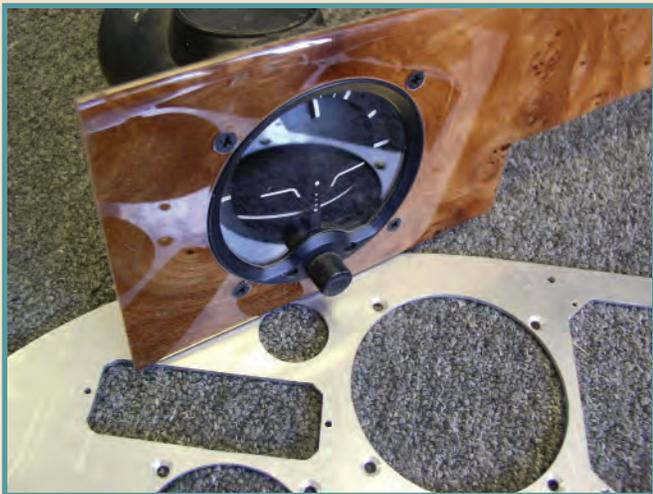
Wood-veneer finished and ready to be mounted to a metal panel.
