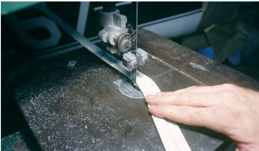
Inner portion of an enhanced-thickness window retainer frame being trimmed on a bandsaw.
