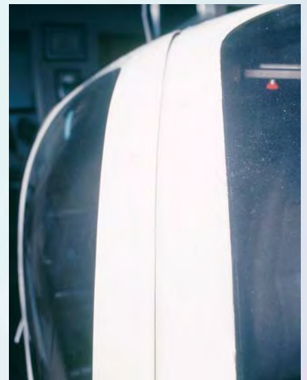
Misaligned cabin doors caused by improperly trimmed windshield being forced into its structural frame.
