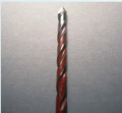
Special tip of Plexiglas drill bit.
