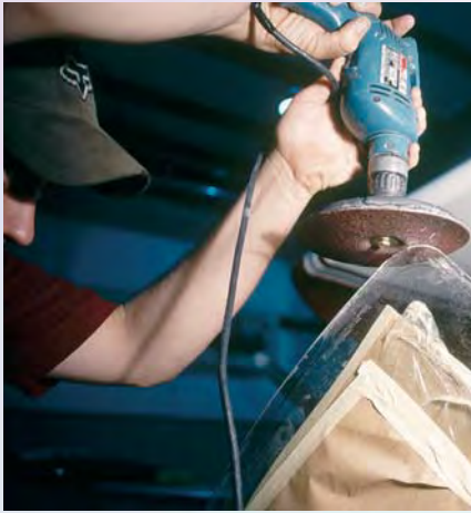
Edge of an acrylic window being trimmed with a disc sander.
