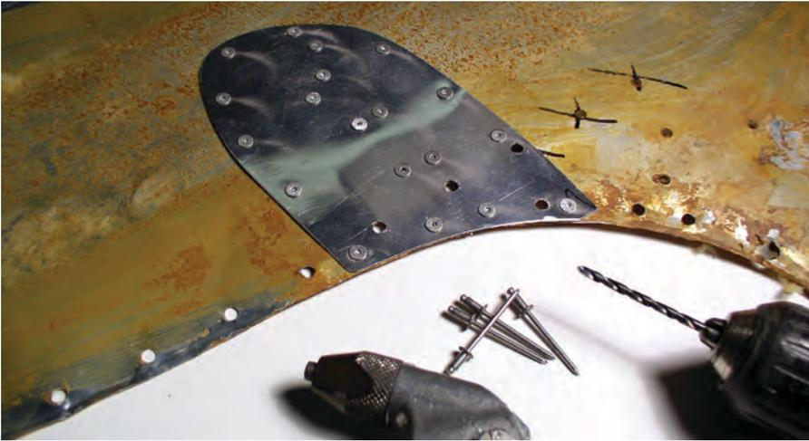
Typical torn aluminum panel repair.
