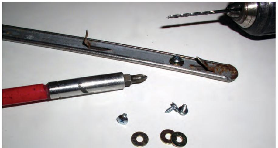
These #4PK screws and washers hold better than the original delicate mounting tabs.
