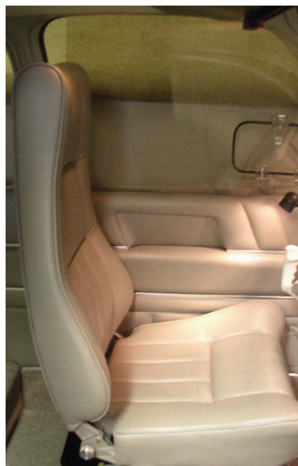
All aluminum rail-mounted side panel installation in a 1950 B35.
