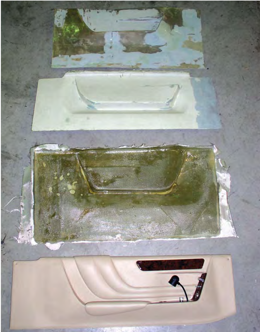
Four-step process to fabricating a fiberglass side panel. Top to bottom: (1) Handbuilt prototype side panel, (2) epoxy mold, (3) rough-formed glass side panel, and (4) trimmed fit and upholstered side panel.
