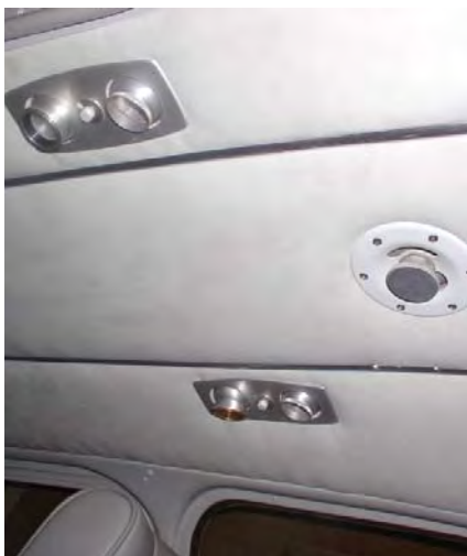
Rail-mounted three-piece headliner with overhead lights and air vents in a B35.
