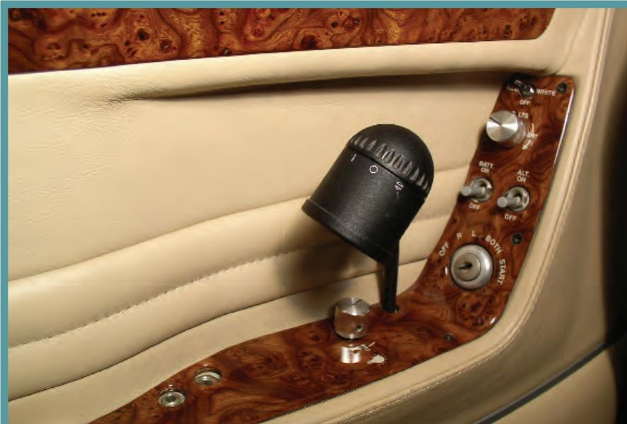
Typical gooseneck light and dimming rheostat installation in the pilot's armrest of a G35 Bonanza.
