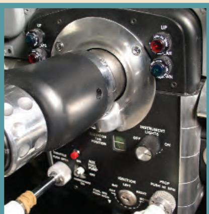
New Dialco front serviceable dimmable gear and flap indicator lights.
