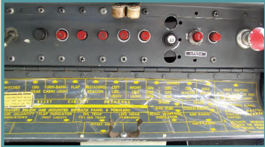
Non-pullable original circuit breakers in an M35.
