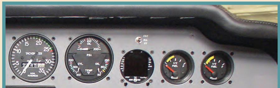
New Mitchell fuel gauges and AIM 3-in-1 oil pressure, oil temperature and cylinder-head temperature gauge.
