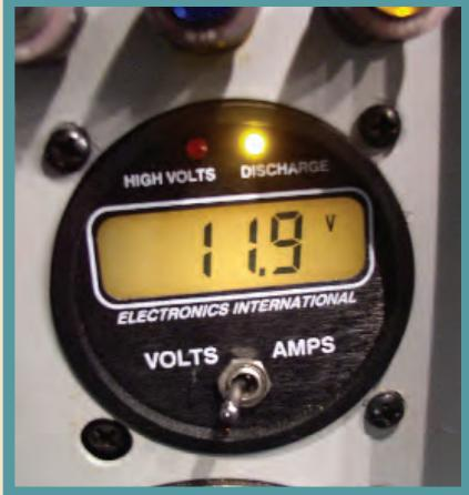
Electronics International VA1A digital volt amp meter with warning lights.
