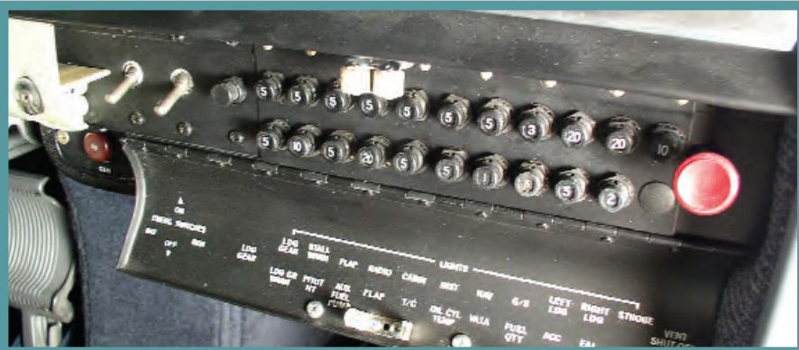
Re-worked circuit breaker panel with pullable Klixon mini circuit breakers.
