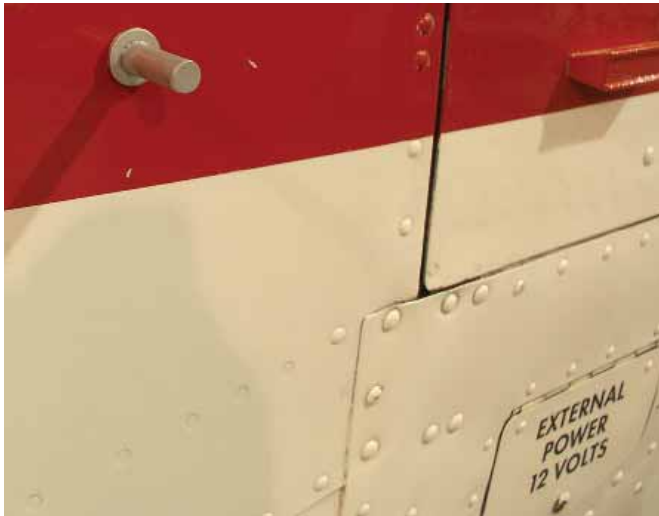
Probe for an electronic OAT, mounted on boot cowl area between cowling and cabin door.
