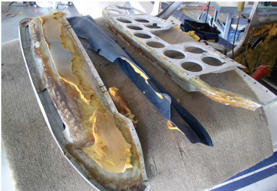
Old, permanently-mounted glareshield and defroster assembly.
