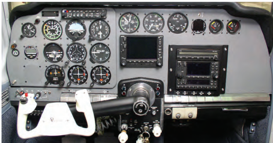
Option 3: Taller "piano-keys up" panel mod with the larger three-row shock-mounted flight panel and a center-mounted multifunction display.
