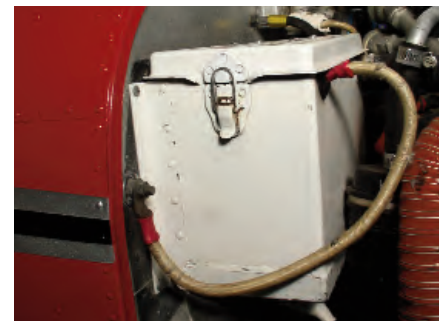
New battery box mounted on forward side of firewall.
