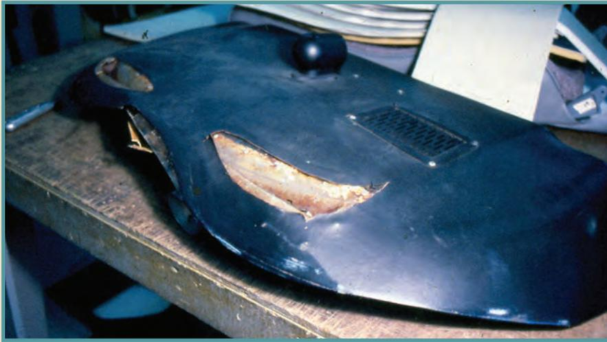
A 12-year-old factory glareshield destroyed by a shrinking and deteriorating leather cover.
