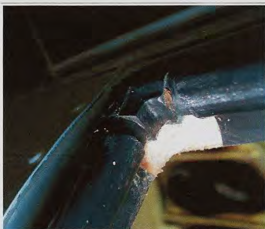
30 years of time has caused the corner piece to shrink and separate.
