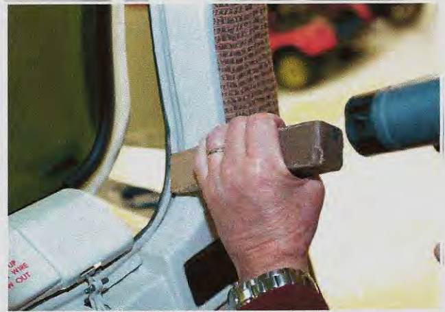
Leather-tipped wood drift and hammer re-forming the flange of the opening window.
