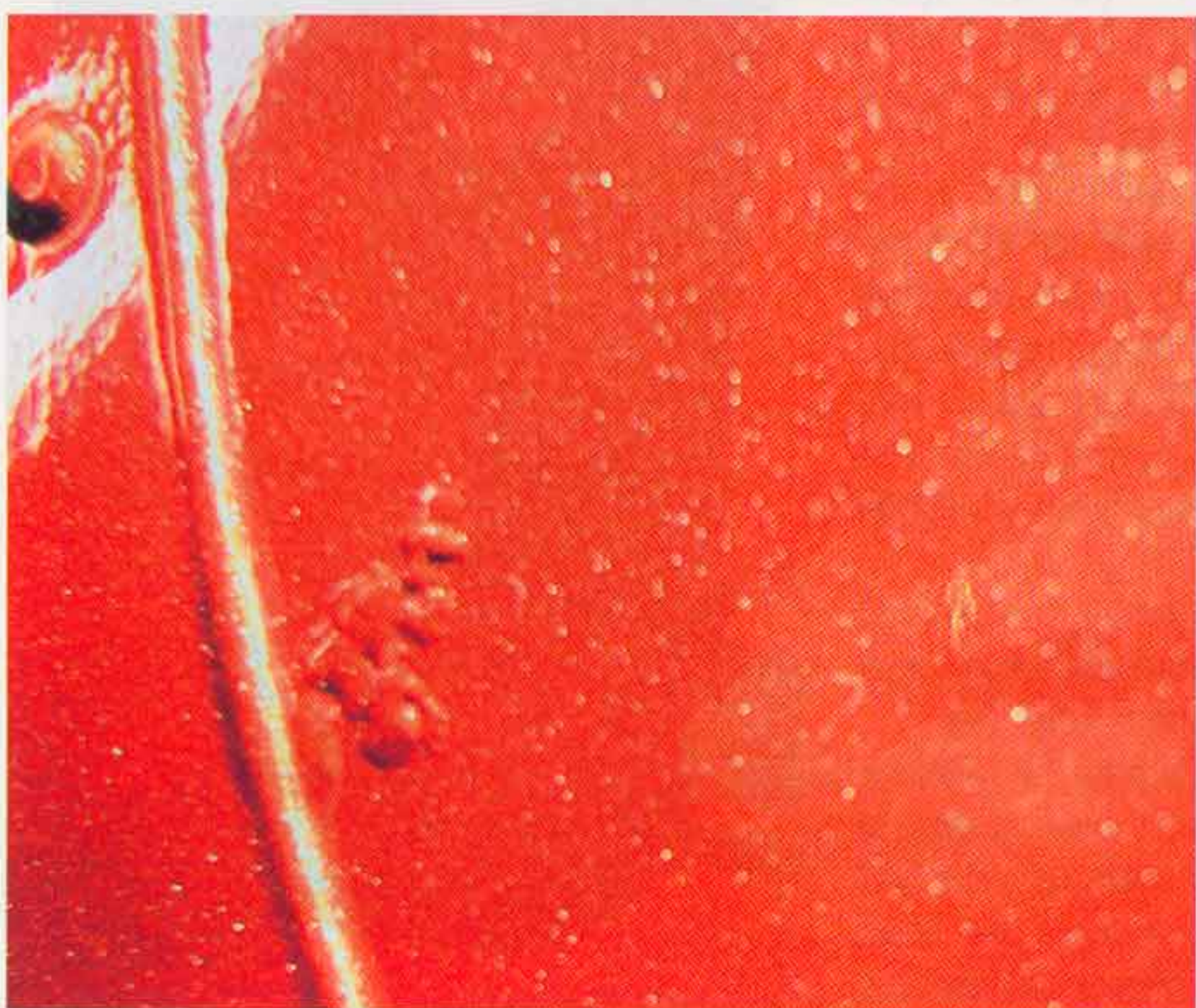
Figure 3—Early stage of filiform corrosion. Notice irregular swelling caused by corrosion trapped under the paint.
