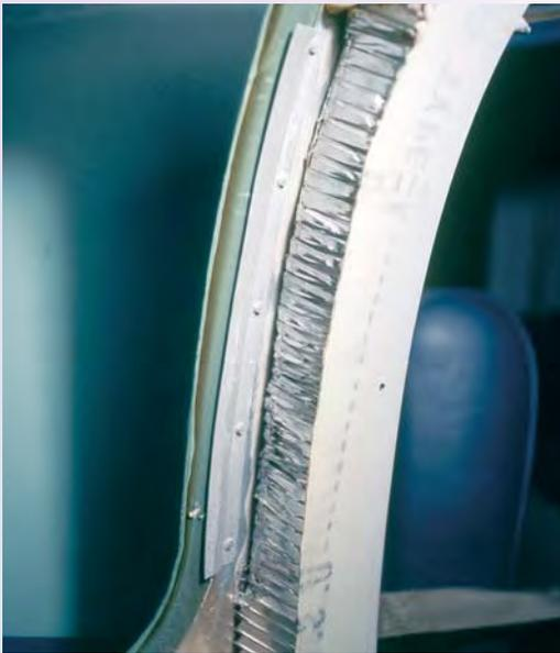
(3) Forked inner frame mounted window in an A36 cargo door shows the 3/32" (on center) flush rivets holding the inner frame snugly against the window.
