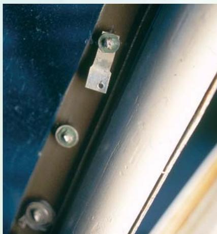
(5) Direct structural mounting method showing 1/4" holes drilled near the window's edge. Mounting hardware and sealer can also be seen in this photo.
