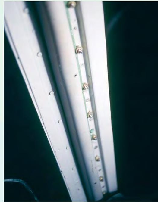
(1) Original frame-type installation showing shake-proof nuts holding the framed windshield assembly in place.
