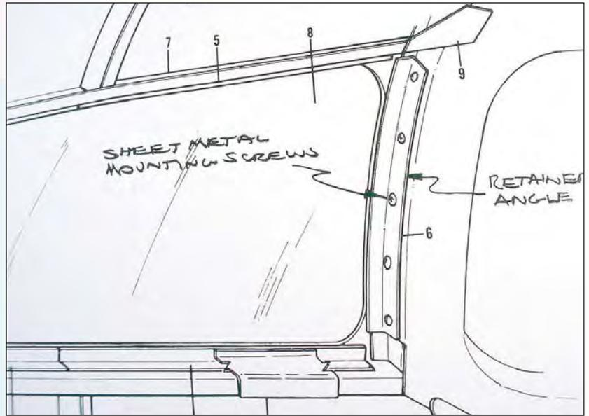
(4) Long third window mounted with all internal angles and screws—no hardware through to the outside of the airframe.
