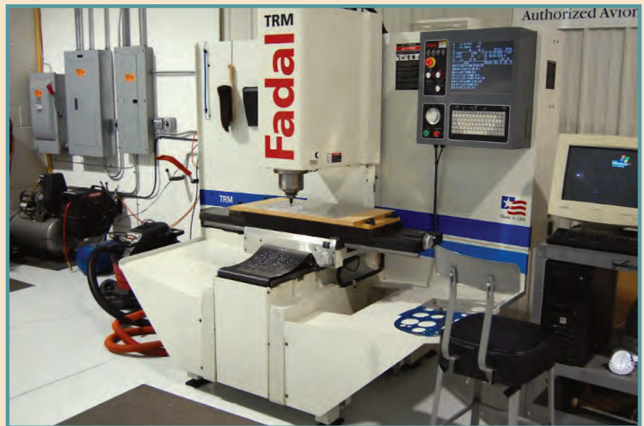
The NC milling machine at Cincinnati Avionics cuts very accurate instrument panels and holes.
