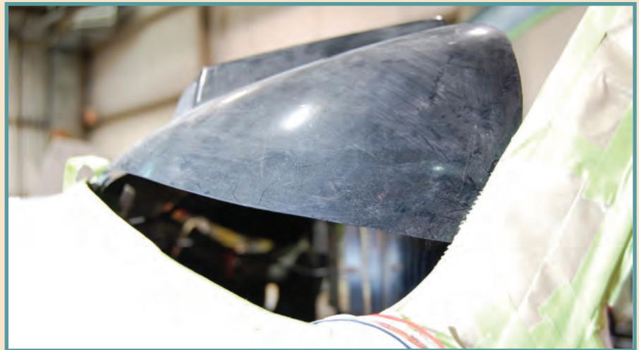
Not enough clearance for the glareshield and the non-sloped windshield.
