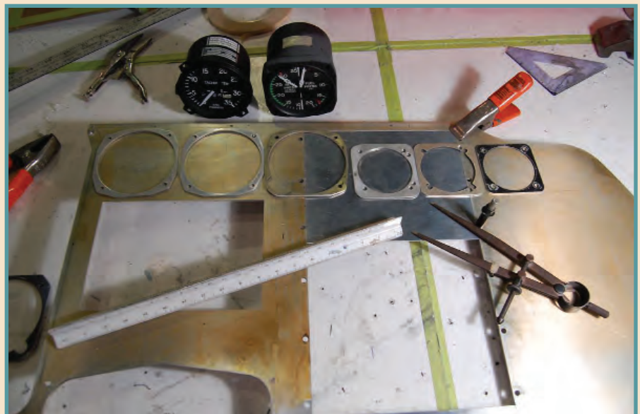
Using precision cut instrument patterns to accurately lay out the fixed panel.
