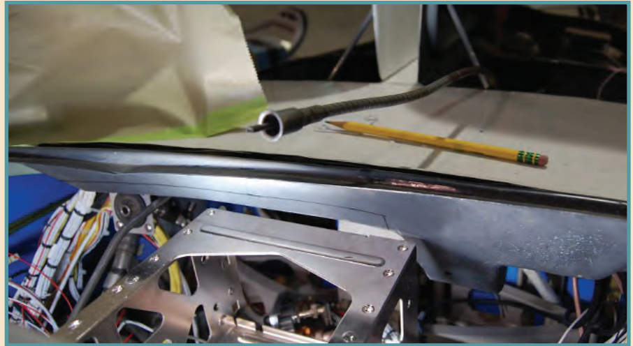
Limited clearance between the upper fixed panel and the original windshield frame.
