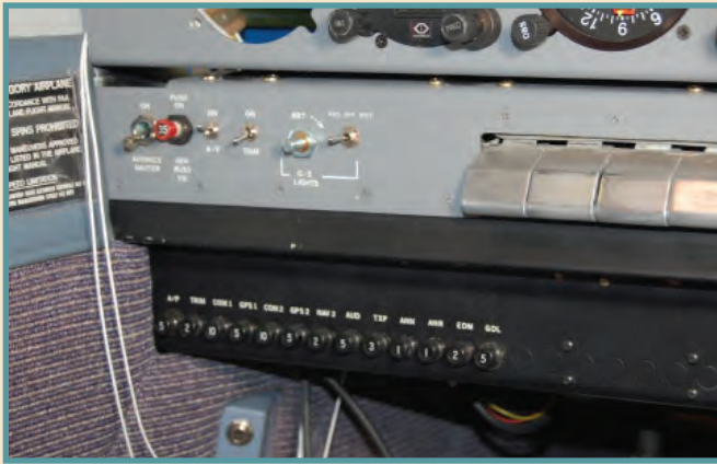
Primary radio and glareshield lighting controls and avionics breakers.
