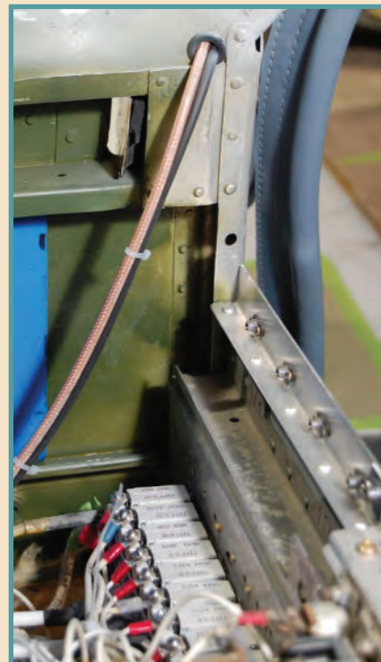
Copilot lower panel mounting angle and nut plates.
