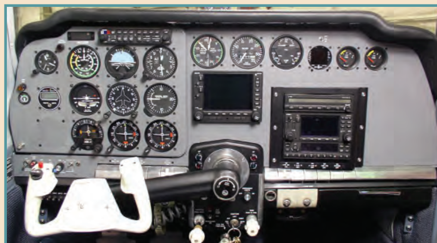
The full height D'Shannon panel, cut to accommodate original piano keys and center throttle quadrant.
