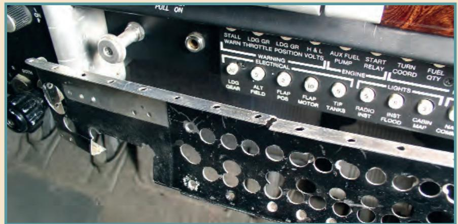
An example of a poorly designed and fabricated subpanel truss that had failed in service, allowing the center throttle quadrant to move about 1/8" vertically.
