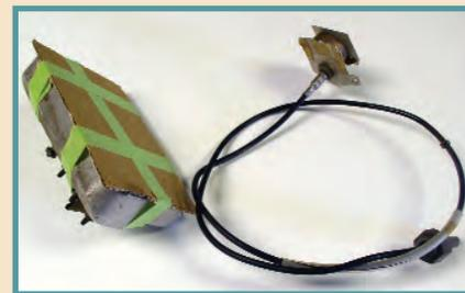
Properly protected engine and fuel gauges.
