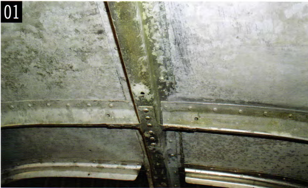
Corrosion found on the cabin top of a 1976 Cessna 172.
