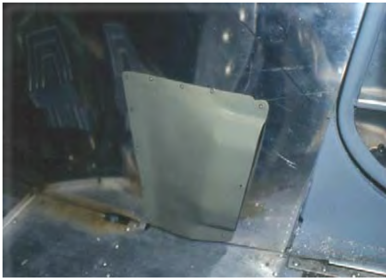
New .025" aluminum side panel with the re-located original heat outlet cover riveted in place.
