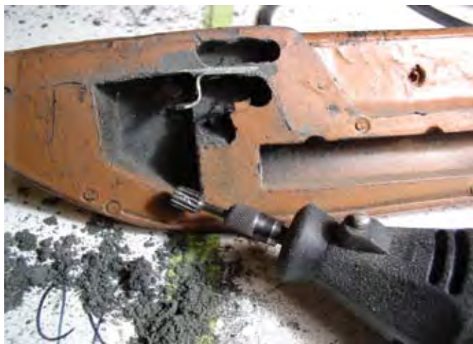
The old foam is easily removed with a router bit and a moto tool.
