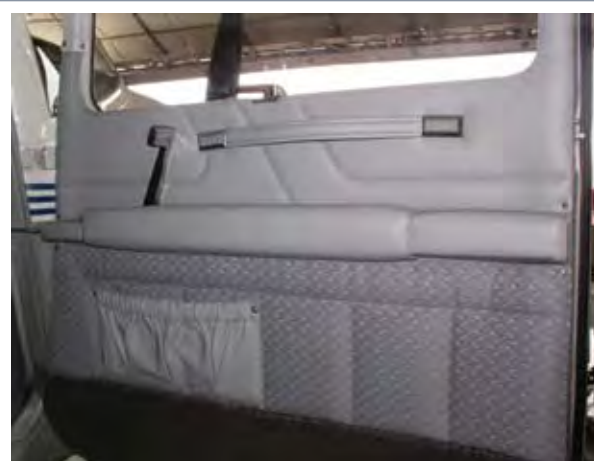
The same armrest with the dented aluminum overlay removed, and the entire assembly covered in leather.
