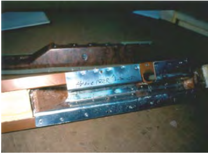
Typical riveted aluminum reinforcement - very strong!
