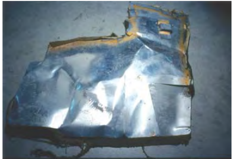
Original forward side panel removed from a 182. The condition we see here is typical.
