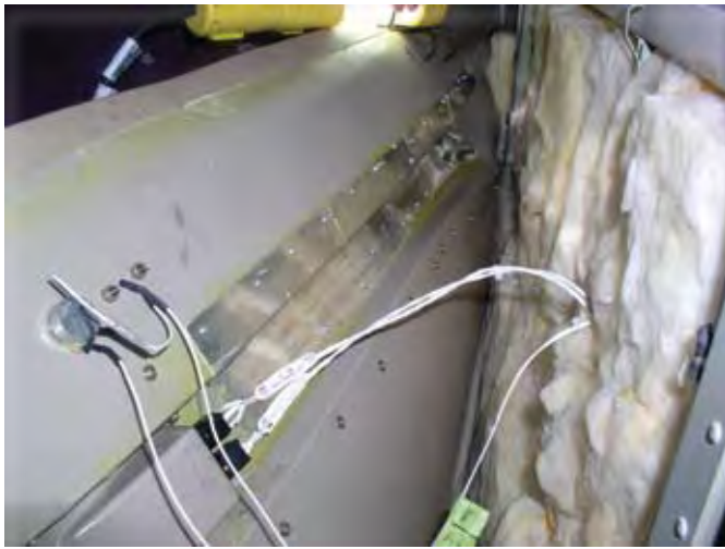
Aluminum reinforcement on a vacuum formed armrest (this component had cracked after only 100 hours in service).
