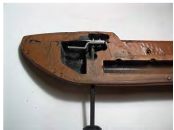
The new steel tab being installed with machine screws and nuts. Note the access holes that we drilled through the rubber base to facilitate installation of the mounting screws.
