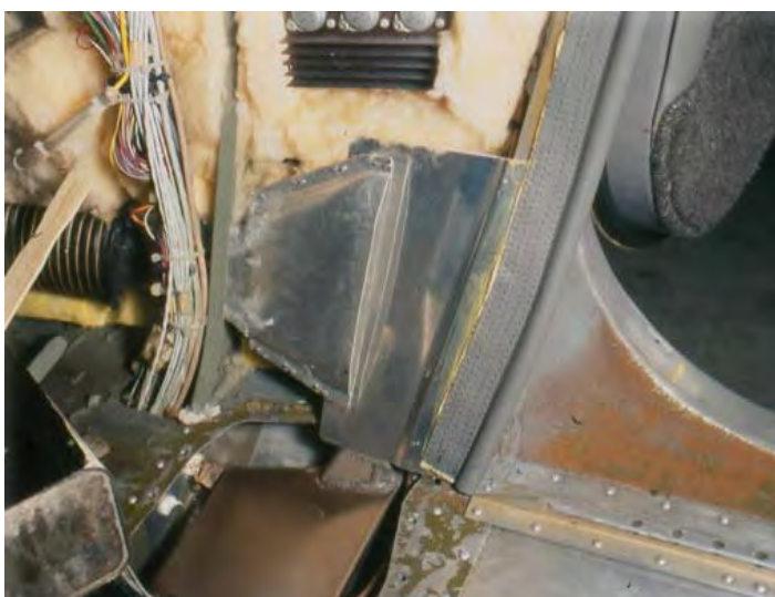
Heat outlet, re-trimmed and mounted 2" forward of its original location
