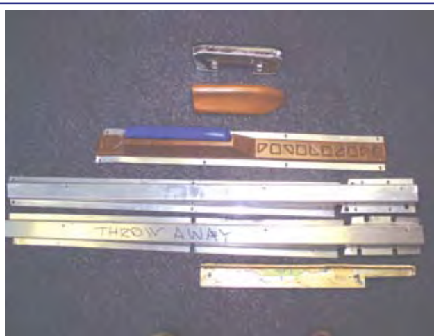
From top to bottom: 60's injection molded, 70's rubber molded, late 70's-80's composite, and 70's 210 all aluminum (three pieces - center one is discarded).
