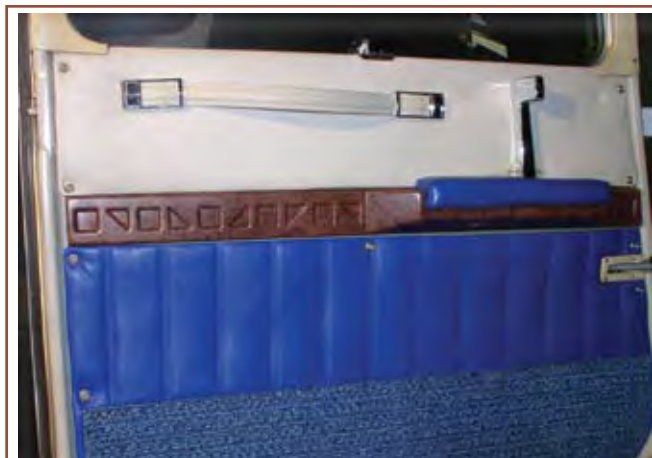
Original factory finish-out for the 80's composite armrest.
