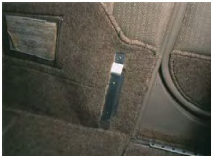
Re-designed and relocated heat outlet
