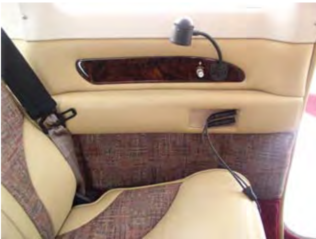
A new 206 done in our shop, with reinforced and upholstered side panels
