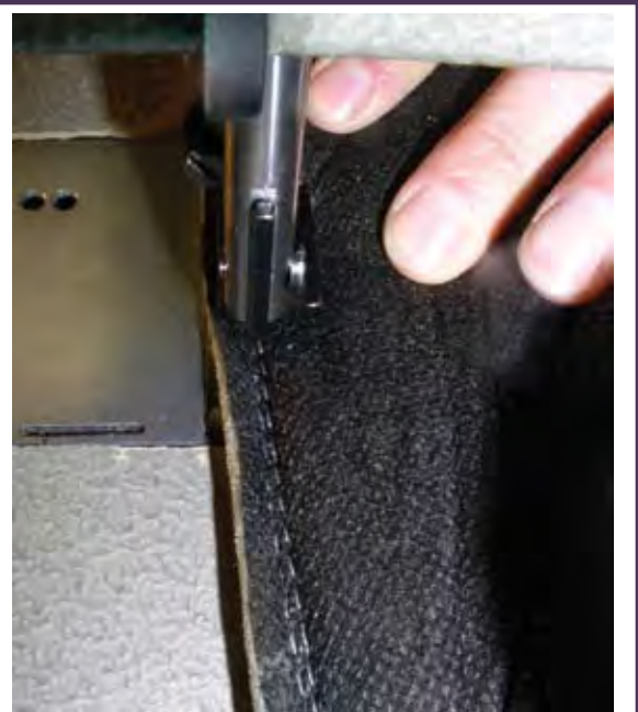
Eight Layers of finish material, backing foam, and fabric. Note the nice wide stitches - strong and durable.
