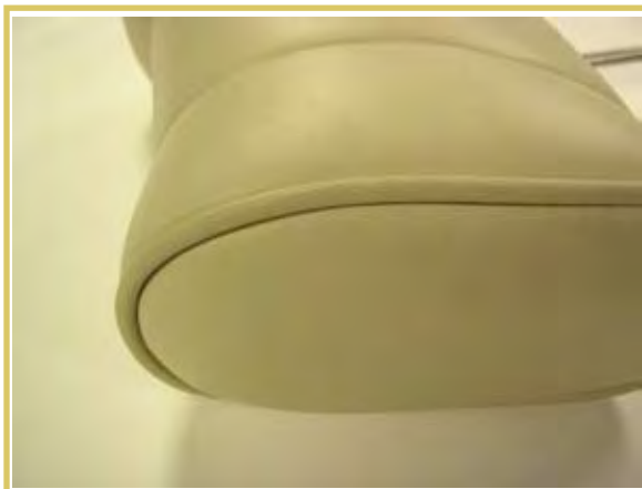
Corded seam. Looks good, wears well and is replaceable.
