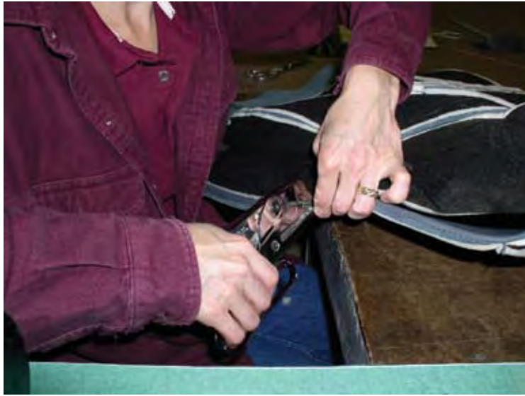
Temporarily staple the seat together to help hold the panels during the sewing process.
