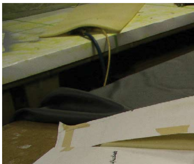
Patterns being fabricated on a Cessna seat back.
