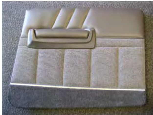
.125" Lustran vacuum-formed armrest for an early 150, 152, 170, 172, 180, 182, 185, 205, 206 or 210.
