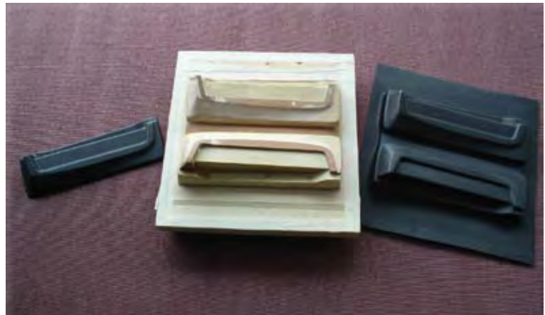
Finished armrest (left), wood mold (center), and untrimmed formed armrests (right).
