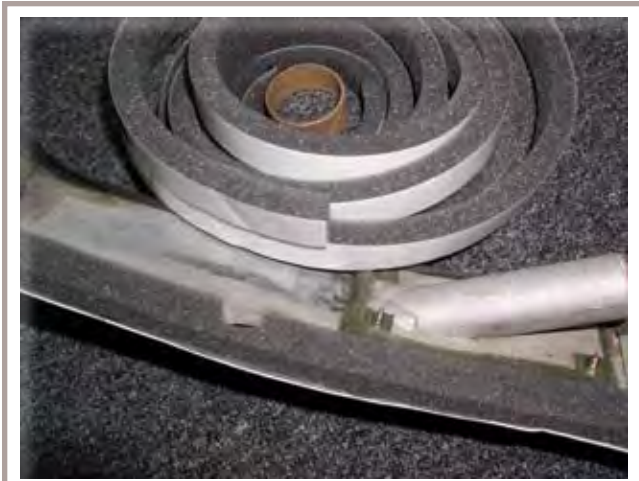
Soft foam weatherstrip seal applied to removable wingroot fairings.
