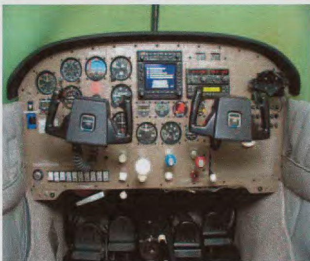
A great avionics package and well built all-metal instrument panel with new switches and circuit breakers
