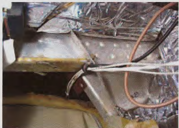
Super-clean forward spar attach fitting – typical of this entire airframe
