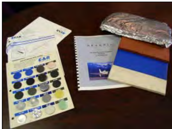
Frequency- and amplitude-specific materials as supplied in the Skandia kit, which comes with a very well written installation manual.
