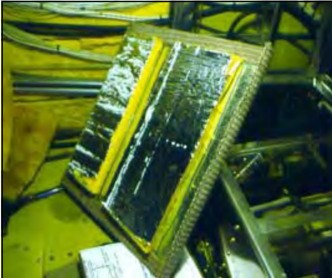
It's important to apply both damping and attenuating materials to the back side of the aft bulkhead access panel.
