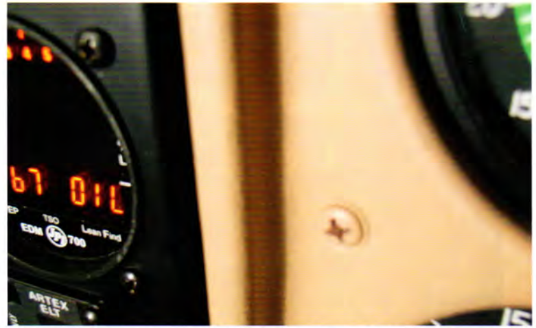
Painted finish screw and washer. Looks good, holds firmly and is easy to install and remove – wow!
