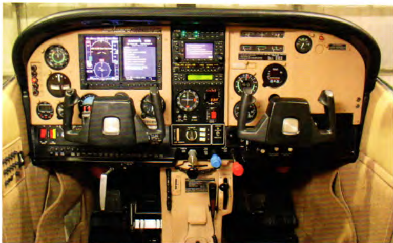
Cosmetically renovated 210 panel, modified to accommodate a Garmin 500 system and more.
