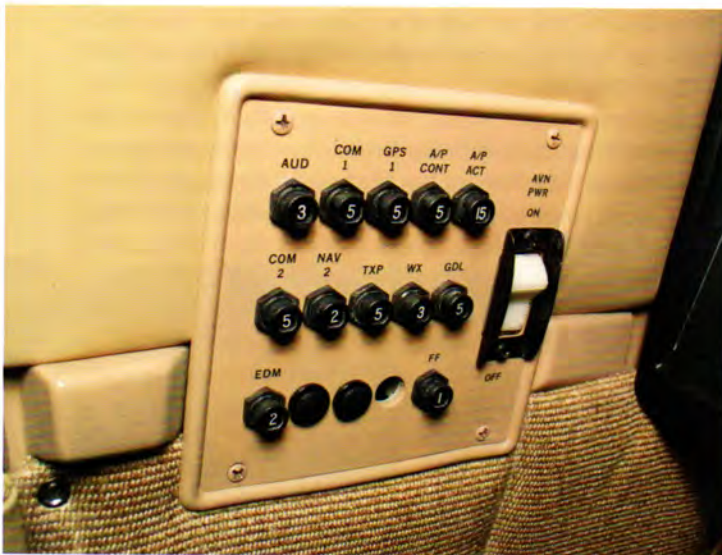
Renovated side panel circuit breaker panel.
