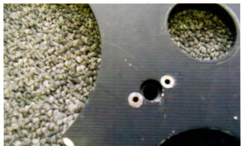
An 8-32 nutplate installed in an oversized hole.
