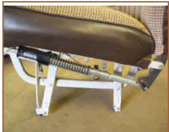
Hydrolock type of reclining mechanism - great system!
