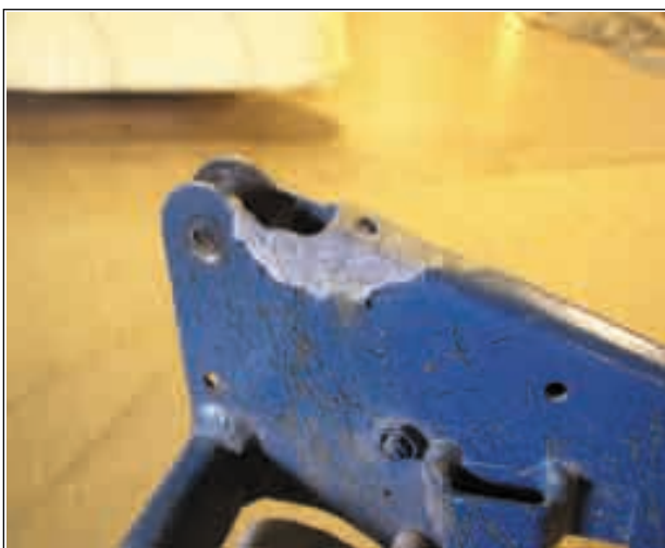
Seat back attach point compromised by severe corrosion
