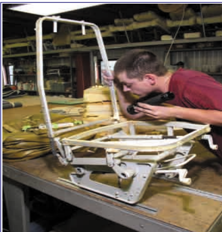
Checking seat frame and mechanisms (this can also be done in the airplane).
