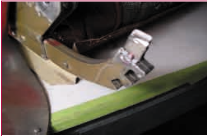
Damaged reclining cam
