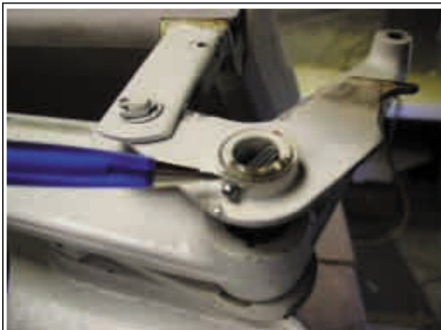
Point of frequent cracks in reclining bellcrank
