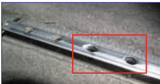
Worn seat track stop hole
