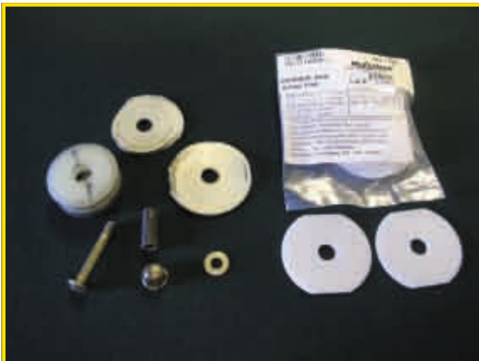
Old thrust washers on left, new teflon washers pictures at right.
