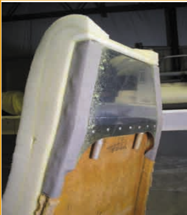
Riveted natural seat back build
