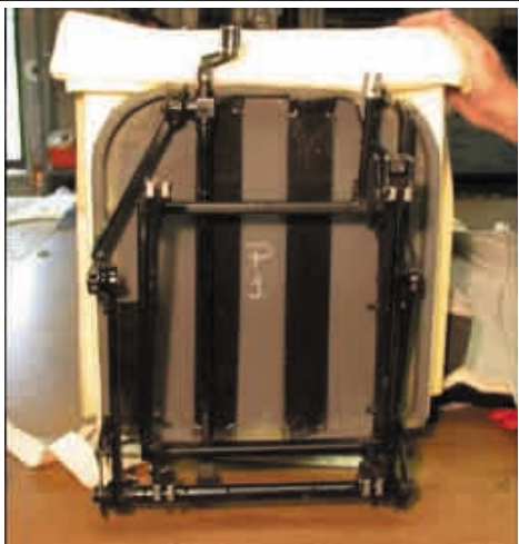
New seat sling with strong seatbelt webbing reinforcement - good forever
