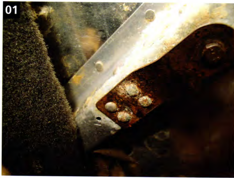
Many older airframes exhibit corrosion, but it often can be mitigated.
