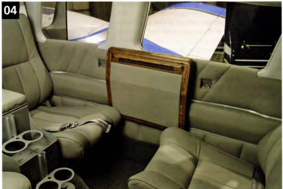
Composite side panels with recessed armrests are one of many optional upgrades available when renovating a Piper interior.
