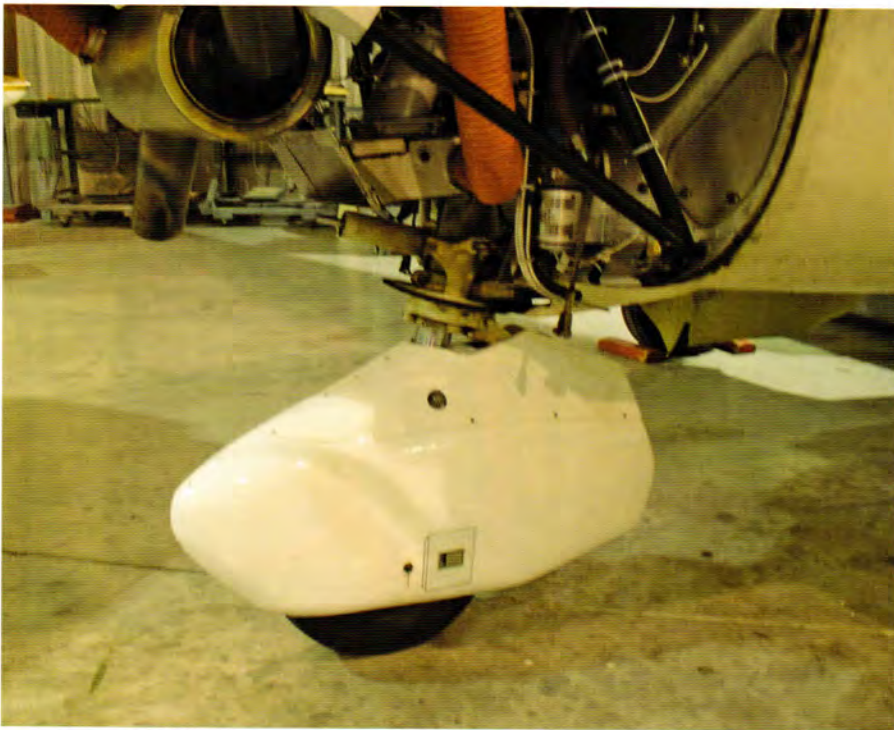
Speed-enhancing full nosegear fairing.
