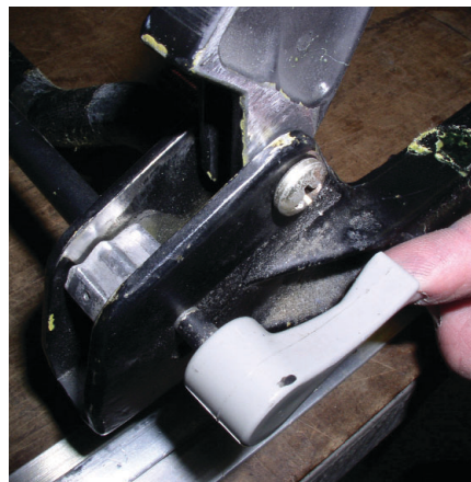
Current production three-position cam type seat reclining mechanism very reliable.
