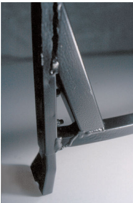
Repaired seat frame weld with a gusset added to prevent another failure in the future.
