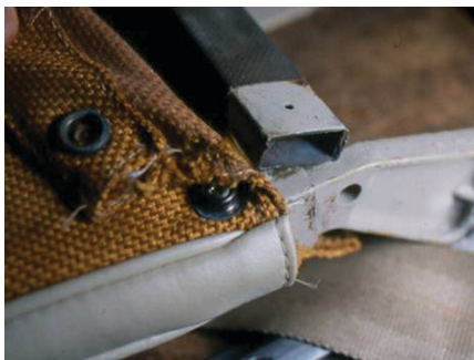
Seat back bottom tube completely broken away.
