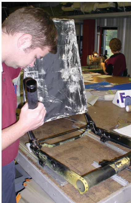
Seat frame being checked on bench-mounted test rails.
