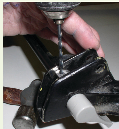
This is an easy way to remove a broken roll pin.
