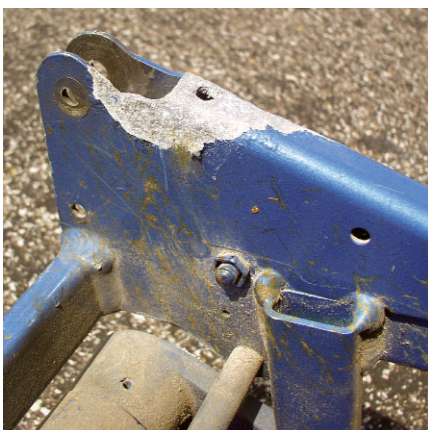
Corroded seat caused by post-tanning flame-proofing.
