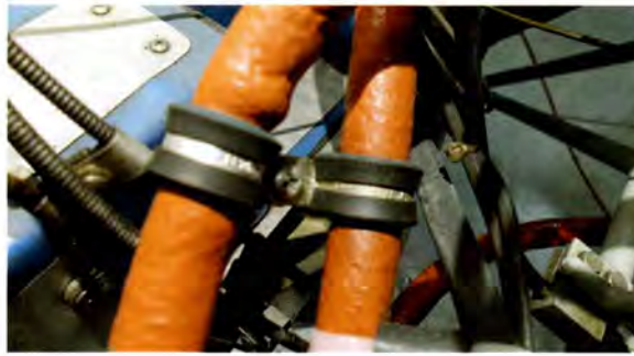
The correct use of two rubber-shielded Adel clamps, secured with 10-32 stainless steel machine screw and a self-locking nut.
