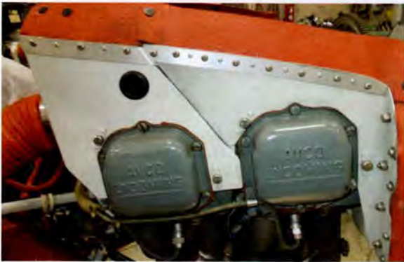
Scotch-Brite pads for surface prep, SEM Self-Etching Chromate Primer and acrylic professional baffle finish.
