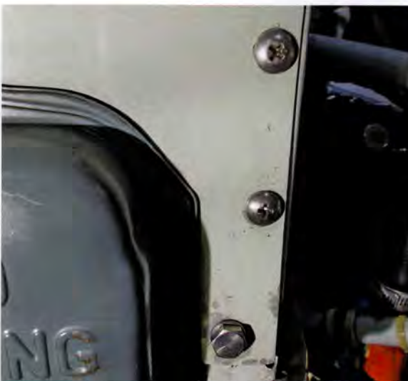
Non-structural stainless steel machine screws, holding two baffle sections together.
