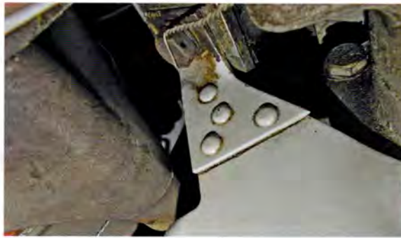
Mounting bracket repair, secured with bucked aircraft rivets.
