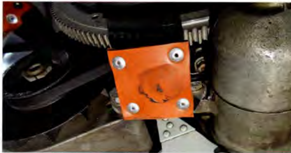
Silicone rubber bumper pad, secured with non-structural Marson pop rivets.
