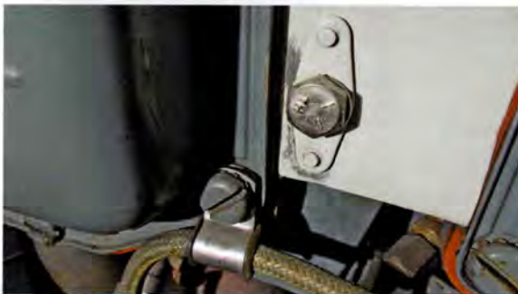
Non-structural stainless steel bolt, securing a baffle to a cylinder head.
