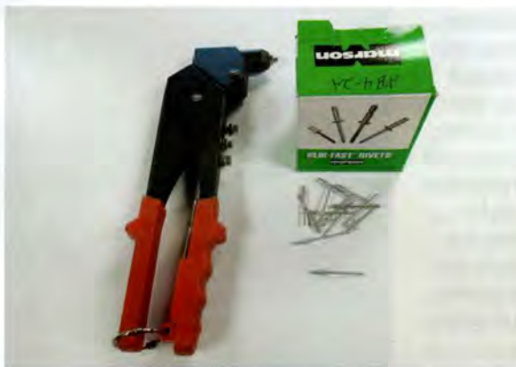
A rivet puller and 1/8-inch non-structural Marson rivets, used to repair baffles.
