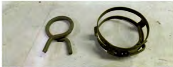
At left: a less-reliable spring clamp. At right: ratchet clamp.
