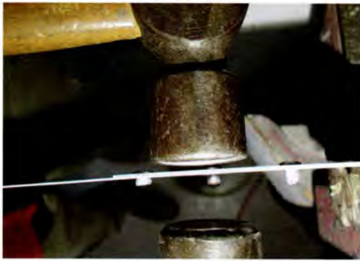
Use two hammers to more tightly set a pulled Marson pop rivet.
