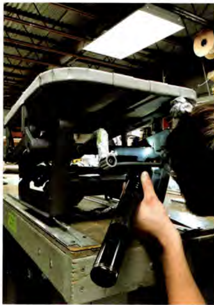
Certificated aviation maintenance technician thoroughly inspecting a seat for structural and mechanical condition.
