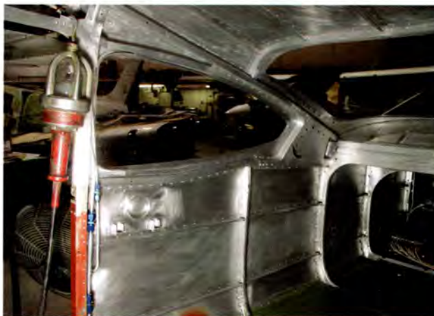
Cessna 182 thoroughly cleaned and ready for application of corrosion-inhibiting zinc chromate.
