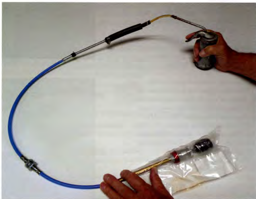
Pressure-lubricating a throttle cable before installation on a new engine.
