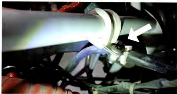
A closeup of the metal locking tab built into high-quality wire ties.
