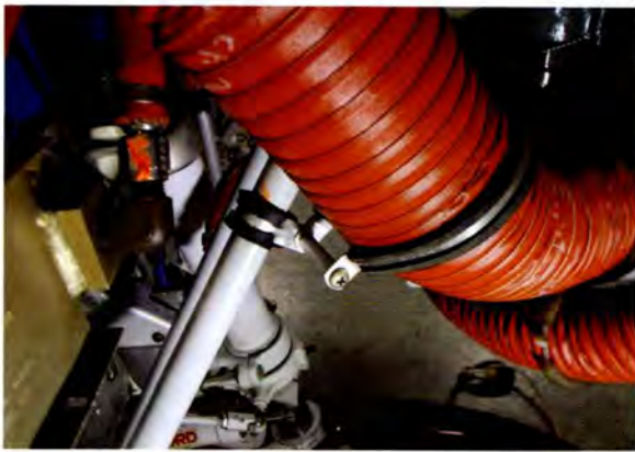
Two rubber-cushioned Adel clamps secure a large-diameter hose to an engine mount.
