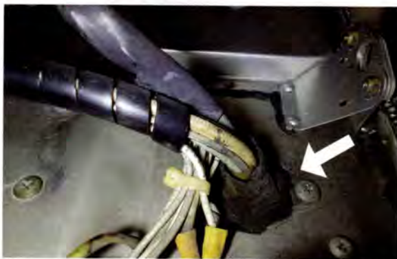
A metal flanged pass-through correctly installed at the factory. This engineered firewall pass-through will actually protect the cabin from smoke and hot gases of an engine fire.
