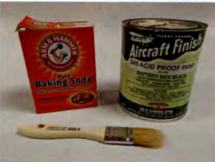
Acid-neutralizing baking soda and acid-proof battery box paint can help in cleaning up an older battery box.
