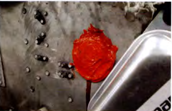
Acid-neutralizing baking soda and acid-proof battery box paint can help in cleaning up an older battery box.
