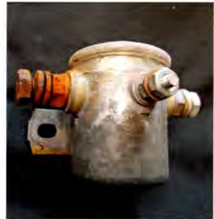
This severely-rusted relay terminal was hidden under a silicone rubber boot.
