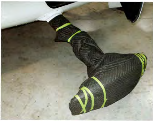
Landing gear protected by a blanket.
