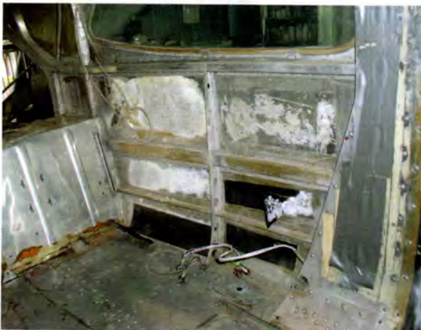
A Cessna cabin after interior removal.
