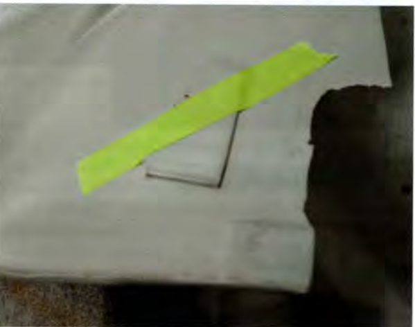
A typical piece of damaged plastic trim; a broken fragment is taped to the larger trim piece for safekeeping.
