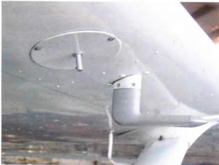
OAT probe mounted in an ideal place on the underside of the wing, shaded from sun, protected by the lift strut and away from any heat source.
