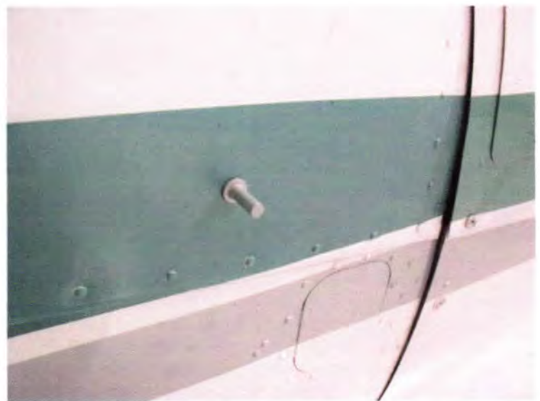
Probe for an electronic OAT, mounted 10" aft of the cowling.
