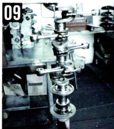
Crankshaft and connecting rods mounted on an engine stand.
