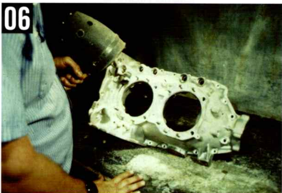
Using a black light to check for cracks in the crankcase.
