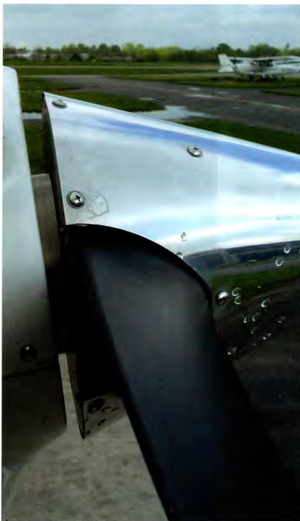
Misaligned propeller spinner indicates old and sagging rubber engine shock mounts.
