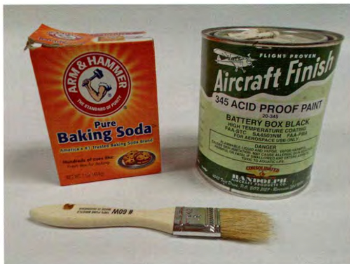
Acid-neutralizing baking soda and acid-proof battery box paint can help in cleaning an older battery box.
