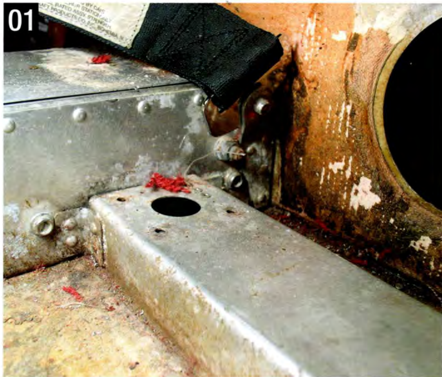
All-too-often-seen corrosion once carpet sections are removed.
