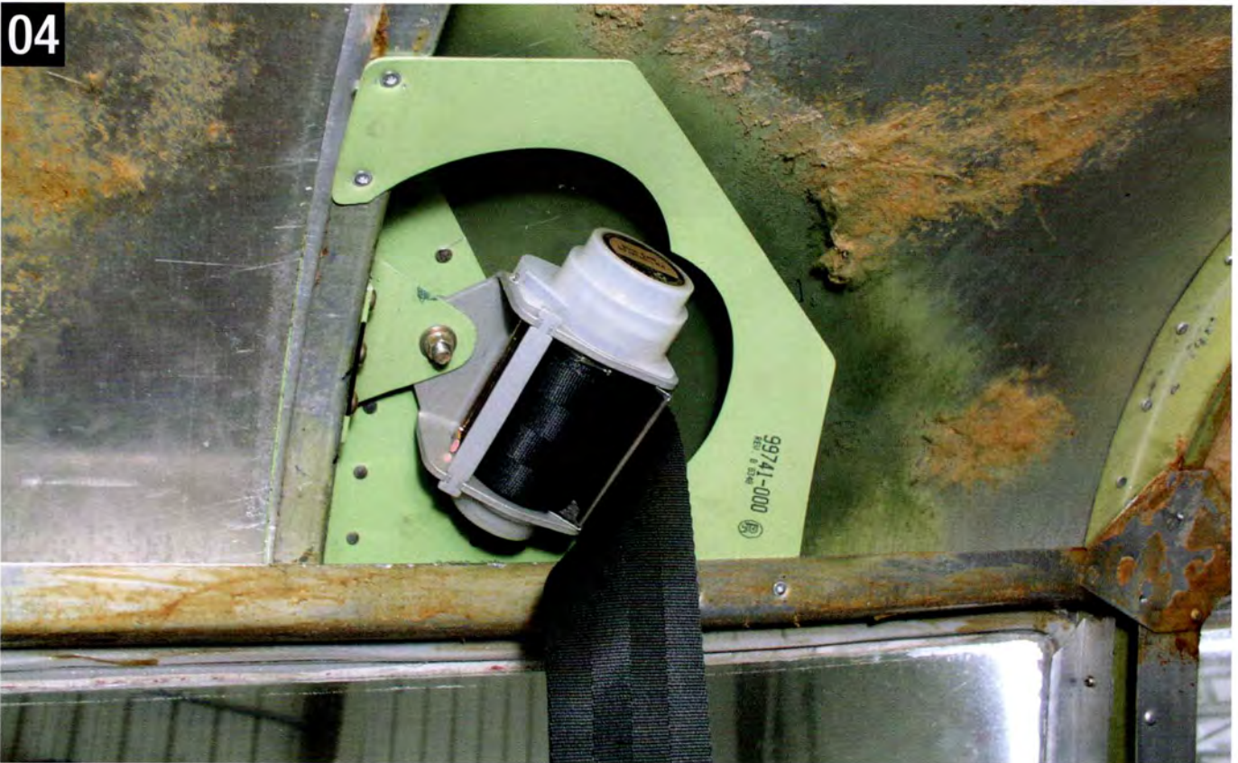
Properly-installed aftermarket shoulder harness bracket.
