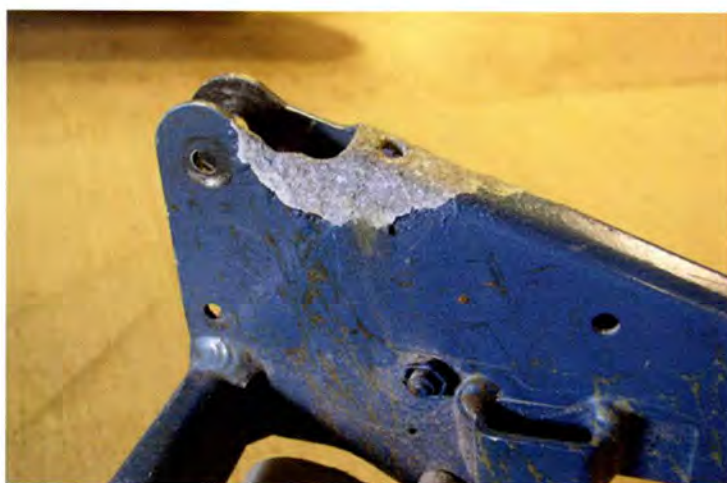
Serious seat corrosion caused by improperly flameproofed upholstery material coming into contact with an aluminum seat frame.
